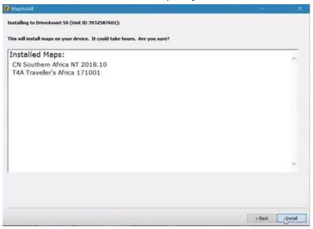
MapInstall will then continue with the installation process. When the installer has completed, click "Finish".
