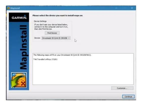
If there is an SD card in the GPS unit, you will notice that MapInstall lists your Device name and the words "+SD Card" - see below. (ie. this means that the T4A maps will be installed on the SD card).
